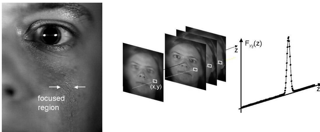
Fig. 3. In the projections of the real image, each slice displays focused and unfocused regions. The evaluation of the focus measure operator F_{xy}(z) for a specific lateral coordinate (x, y) along the z -axis is shown. The z value, for which F_{xy}(z) is maximal, delivers the third coordinate of the focus point.
