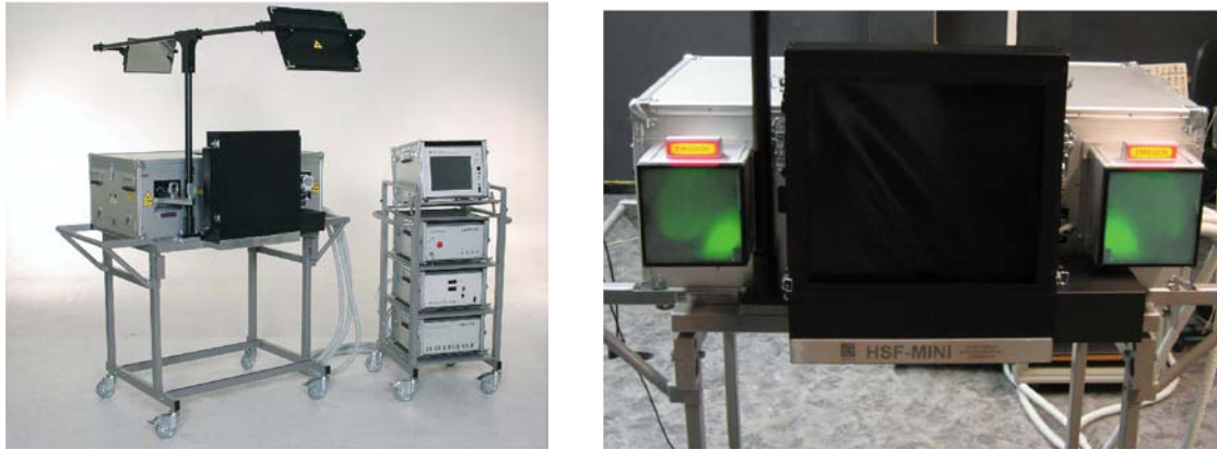
Fig. 1. Left: Mobile holographic camera HSF-mini, developed in cooperation with GEOLA uab (Lithuania). Right: The camera from the viewpoint of the patient. The two illumination ports with the diffuser plates are on the left and right, and the mechanical shutter system that covers the holographic plate is in the center.
