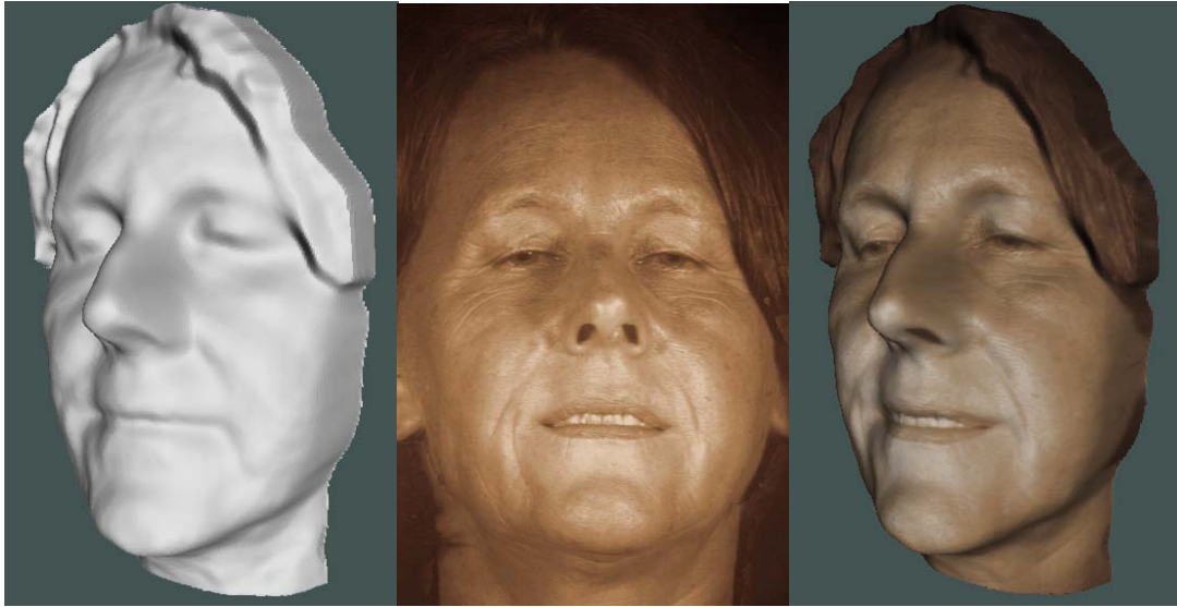
Fig. 4. The textured 3d model is a combination of the surface with the inherent grayscale texture of the hologram.
